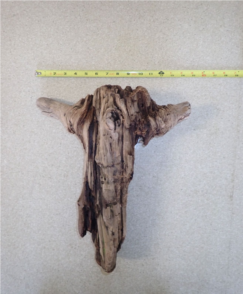
Picture 2: Debris removed from orifice 1A1.
